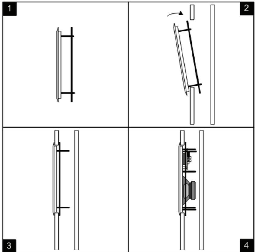
The white frame should fit snugly and smoothly in the cut-out hole. If the hole should have been cut a little too large, the flange on the frame should cover this.
